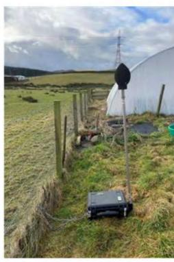
Assuming that this is west of the remote monitoring equipment derivations of the Easterly wind directions may give unusually high readings at higher wind speeds (should the polycarbonate of the polytunnel be loose).
