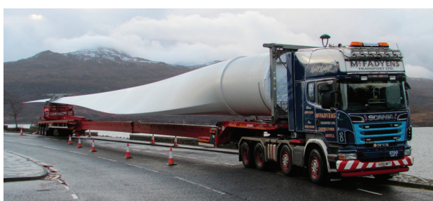
Image: Abnormal Indivisible Load (AIL) Vehicle for Turbine Delivery
